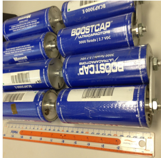
Fig. 3. Energy buffer: 8 series Maxwell BCAP3000 supercapacitors [17].
